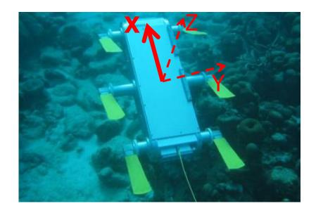
Traditionally the three angles along the axis are called Roll, Pitch, and Yaw
