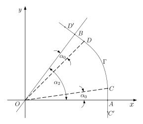
Figure 1: A sketch of the mid curve of the input link of a quasihomokinetic spherical linkage
