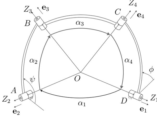
Figure 1: The kinematic chain of a four-bar spherical linkage
