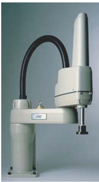
The Adept Cobra 600 is a "best-in-class", four-axis, table-top mounted SCARA robot. Designed and developed in response to customer demand for increased reach, and combined with Adept's easy-to-use software, this robot is an attractive solution for both fixed-automation and manual production methods.
