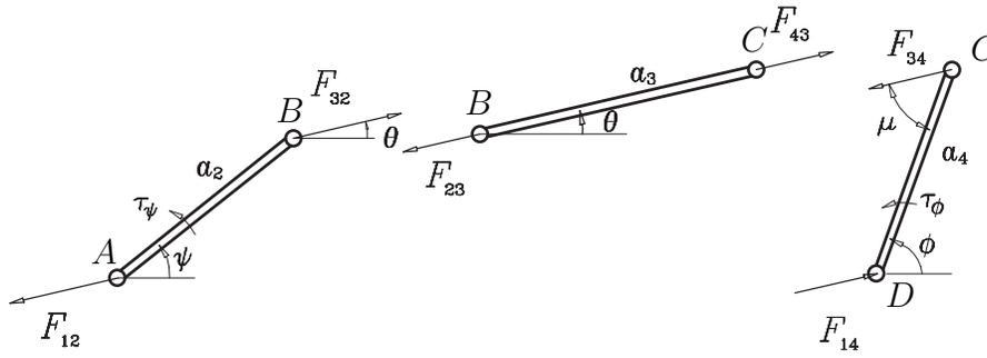
Figure 3.16: A static analysis of the four-bar linkage
