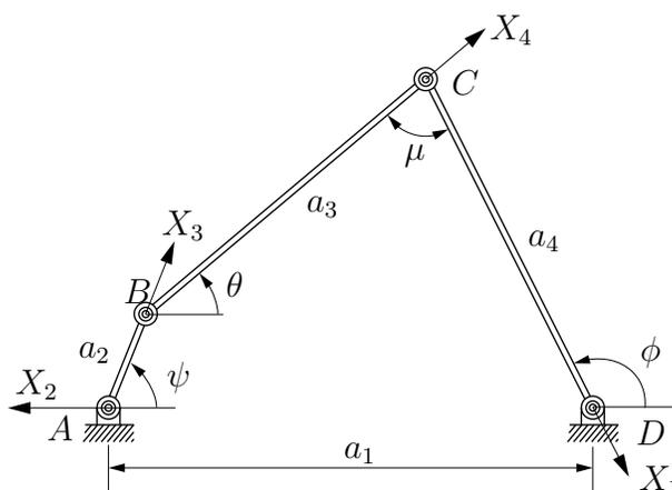
Figure 3.18: A four-bar linkage for function generation
