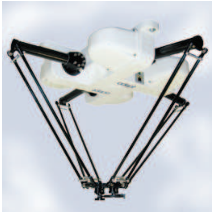
Figure 2.24: Adept Technology's Quattro robot, a parallel Schönflies-motion generator
