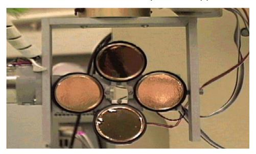
Polaroid sonar emitter/receivers
