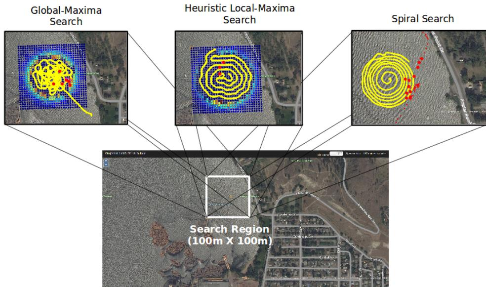
Fig. 7: The search region where field experiments were conducted and the paths generated by three search strategies : Global Maxima, Heuristic Local Maxima, and Spiral Search. Boat’s search path is shown in yellow and drifter’s discrete locations is shown with red dots.
