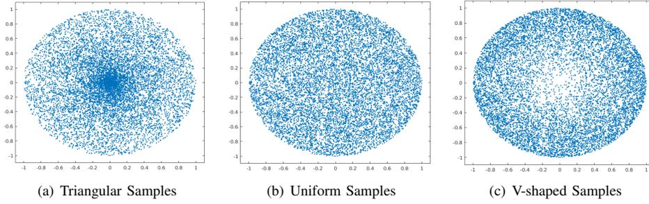
Fig. 3: Samples from three distributions on a unit circle centered at zero. We use these distributions to sample drifter (target) locations for simulating multiple trials.
