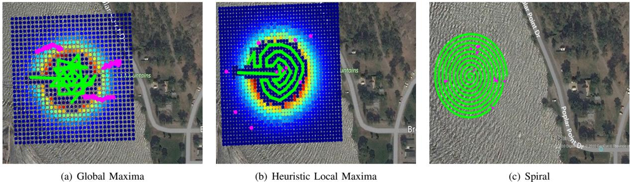
Fig. 2: Simulated global, heuristic local and spiral search paths of the robot (green) and target waypoints (pink).
