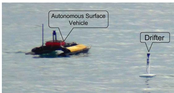
Fig. 8: Autonomous Surface Vehicle, Kingfisher and search target, drifter.
