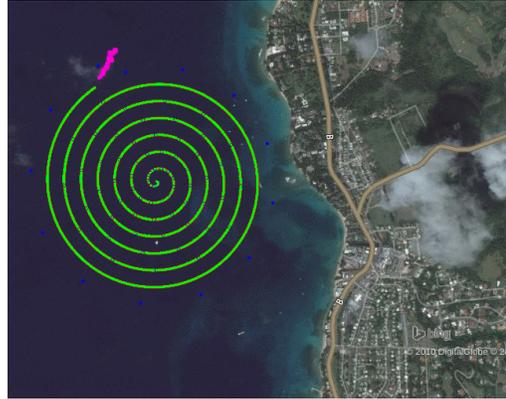
Fig. 1: Simulated search pattern on Microsoft Bing Maps ©. The spiral (in green) indicates the path followed by an ASV terminating at the target waypoints (in pink).
