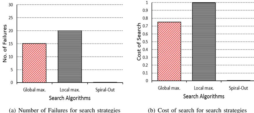
Fig. 6: Multi-target number of failures and cost comparison for different search strategies.
