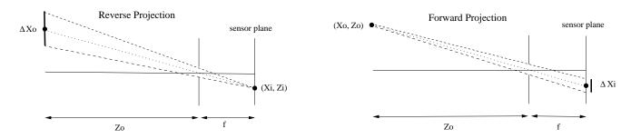
Alternatively, consider the point  $(X_o, Z_o)$  that projects to  $(X_i, f)$  through the center of the aperture, which we take to be the origin. This  $(X_i, f)$  is a single imaged point when the aperture
