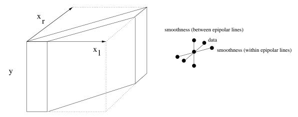
In addition, it is typically unnecessary to use the entire range of disparities. Typical stereo images have disparities from 0 to 50 pixels, with an image width of say 500 pixels. One can use much less memory by using only part of  $(x_l, x_r, y)$  volume, i.e. chopping off the part of the graph which corresponds to larger disparity values. See a sketch above.
