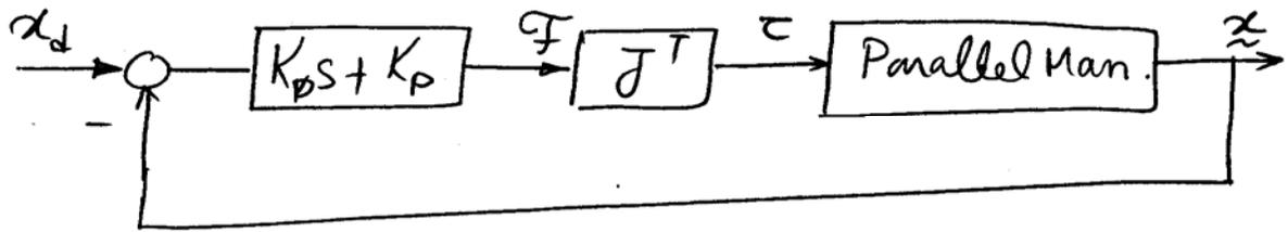
Note that two differences are here from the previous form, one the feedback is  $x$  in task space & the controller output is  $F$  again in task space. In industrial applications even simpler version is used in which
