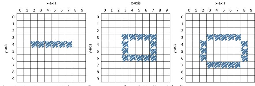
• line (x1, y1, x2, y2) draws a line segment from (x1, y1) to (x2, y2)
