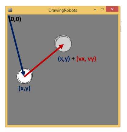
Using the vectors for the Robot and mouse pointer position, we will modify the Robot's velocity
