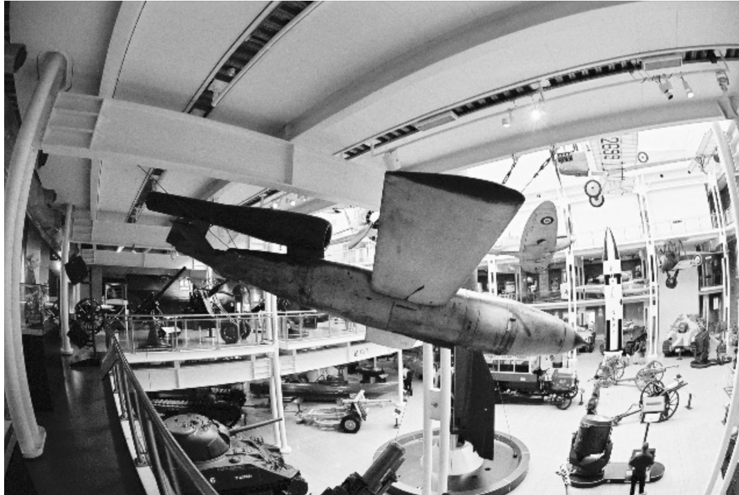
V1 – hanging in the Imperial War Museum, London Built in the 1940's, the V1 could travel over 150 miles autonomously with an accuracy of about 7 miles
