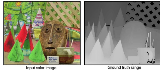
Figure 3: The input intensity image and the associated ground truth range. Since the unknown data are withheld from genuine ground truth data, we can estimate our performance.
