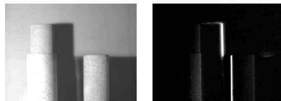
Figure 4: A grey-level image (left) and the difference between successive grey-level images (right).
