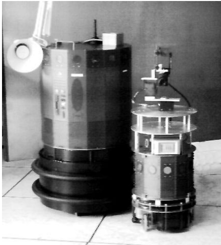
Figure 2: A master robot carries a camera mounted on a pan-tilt unit, and a slave carries a light source. The master moves to a fixed vantage point and remains stationary. The slave then executes a large trajectory about the master.
