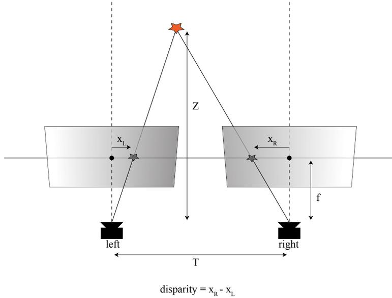
Figure 5: Disparity in a simple stereo system where the view axis of the two cameras are parallel to each other.
