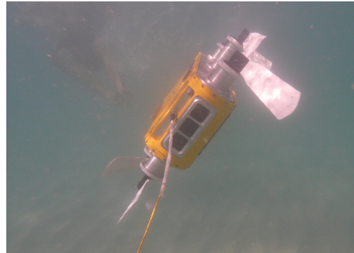
Fig. 2. A tethered Aqua robot performs a 45^\circ turn guided by a PD controller.
