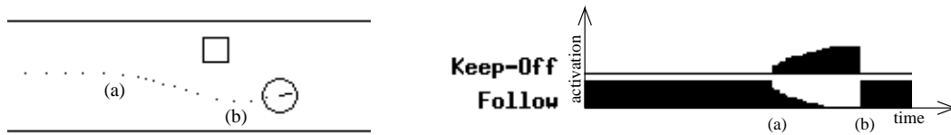
Figure 6: Context-dependent blending of following and avoiding behaviors. After point (a), the Keep-Off behavior starts to become active, and its higher priority dominates the Follow behavior. At point (b), the obstacle is passed, and Follow resumes.
