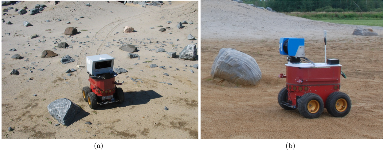
Fig. 2. (a) The ILRIS 3D sensor on top of the modified P2-AT robot. (b) The SICK sensor on a pan-unit mounted on the same robot.
