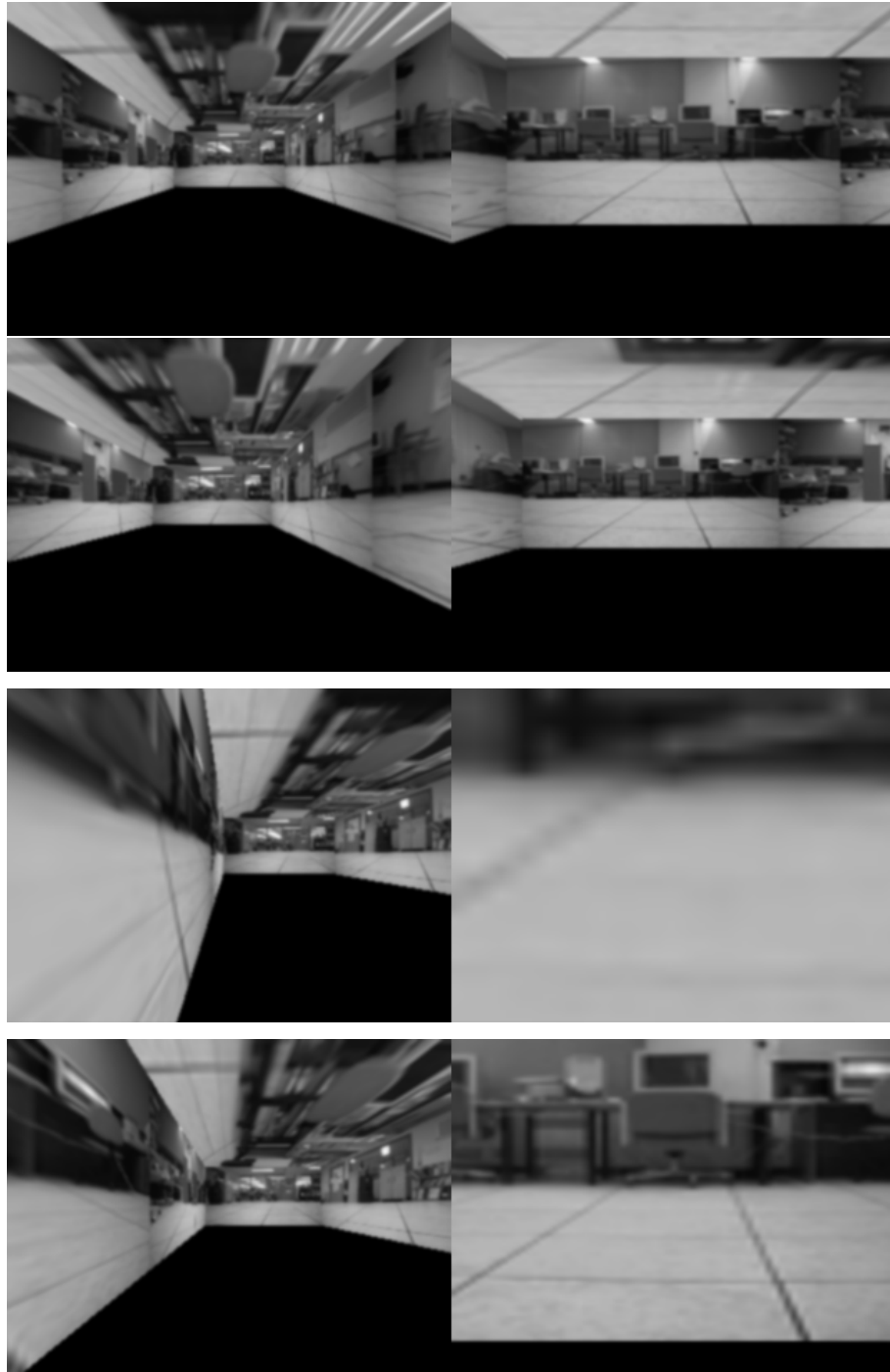
FIGURE 6.3. Example composite observations: A single observation entails acquiring images in two orthogonal directions.
