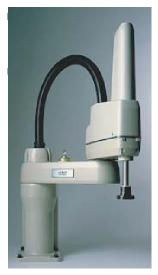
The Adept Cobra 600 is a "best-in-class", four-axis, table-top mounted SCARA robot. Designed and developed in response to customer demand for increased reach, and combined with Adept's easy-to-use software, this robot is an attractive solution for both fixedautomation and manual production methods.
