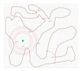
FIGURE 5. The concentric regions indicate the explored area at the time when the number of concurrent rays in increased. This occurs when an obstacle is encountered at a point in the middle of the exploration frontier within an area that was presumed to be a single ray, *ie* at a ray bifurcation.
