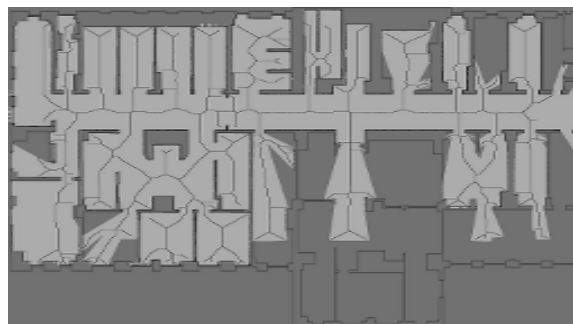
Fig. 2. The skeleton structure overlaid on the grid-based map 1(b) and the floor-plan 1(a)
