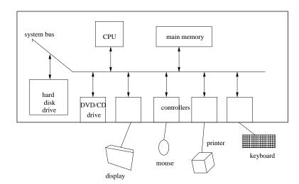
Let's next consider a few examples of how various components can share the system bus. Recall the tri-state buffer circuit element from lecture 6. This was a mechanism for allowing many wires to put signals on a single wire. We will also need to use a tri-state buffers for the system bus. The reason is that we have many devices that can put signals onto the bus, and so only one of them can write to the bus at any time.
