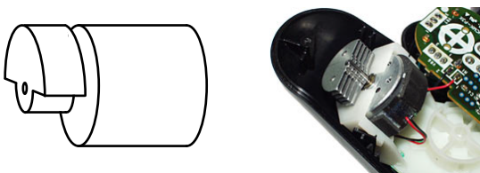
Figure 4: The rumble motor. An eccentric mass spun by a DC motor.
