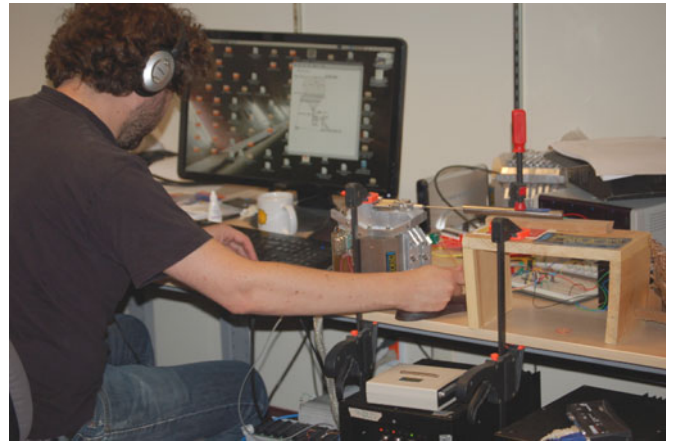
Fig. 6. A participant interacting with the device in experimental conditions. The left hand is manipulating a knob while the right hand interacts with the haptic device. The device is seen in its horizontal configuration, coupled to the velocity transducer.
