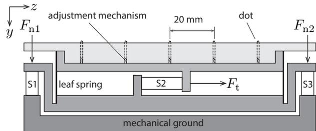
Fig. 1. The apparatus. The transducer measures the interaction forces of the finger exploring the Braille dot platform with dots of adjustable heights.
