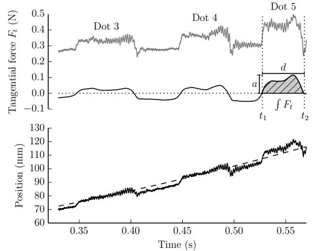
Fig. 3. Recording of a finger exploring three consecutive Braille dots. The duration  $d$  and amplitude  $a$ , defined as  $\max_{t_1 \dots t_2} F_t$ , of the interaction as well as the filtering to measure the friction force integral are shown.
