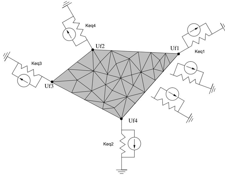
Figure 2: Application of Norton Equivalent to the fine mesh.
