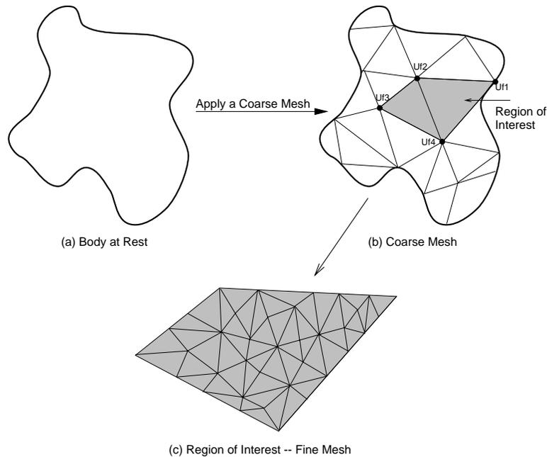
Figure 1: A Deformable 2D Body – Segmenting into Macro and Fine Grids
