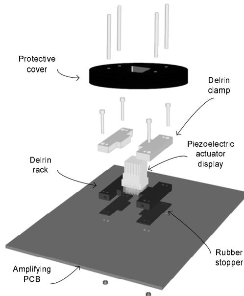
**Fig. 8.** A PCB supports one hundred amplifiers. The outputs are routed via an 8 layer board to a 1 cm<sup>2</sup> pad having one hundred connections. The individual combs are held collectively using two racks and two clamps, forming 10 sockets.
