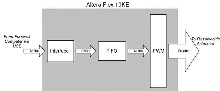
**Fig. 3.** The Flex 10KE is programmed to accomplish three functions: accept serial data from the USB interface, reconstruct images in a first in first out (FIFO) buffer, and generates 100 pulse width modulation (PWM) control signals.
