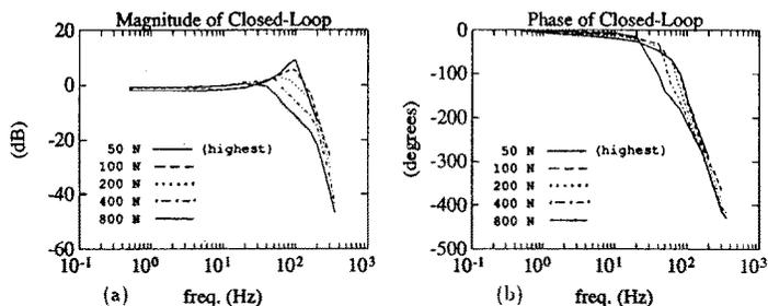
Figure 9: Closed-Loop Frequency Responses: (a) Magnitude, (b) Phase ( $K_f = 2.44$ )
