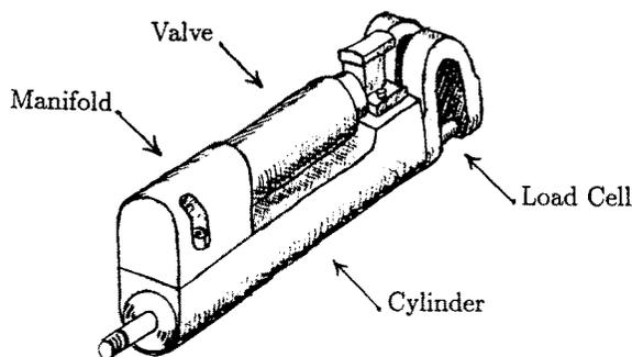
Figure 1: The ASI Hydraulic Actuator
