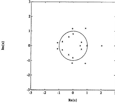
Figure 8: Poles and Zeros of Identified Transfer Function
