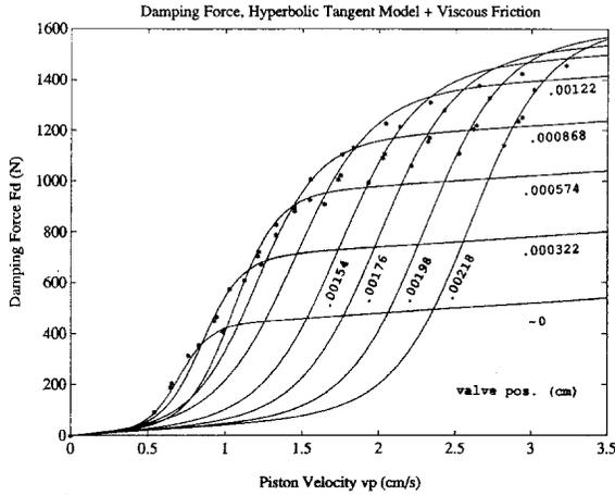
Figure 6: Experimental Hydraulic Damping Effect
