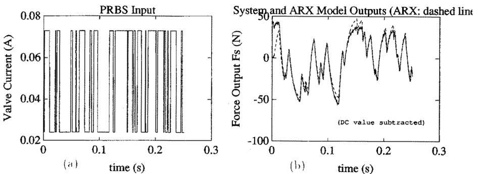
Figure 7: (a) PRBS Input, (b) System and ARX Model Outputs
