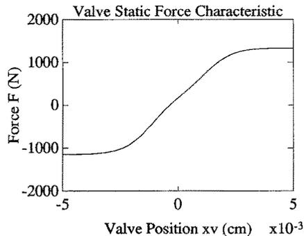
Figure 3: Valve Static Force Characteristic
