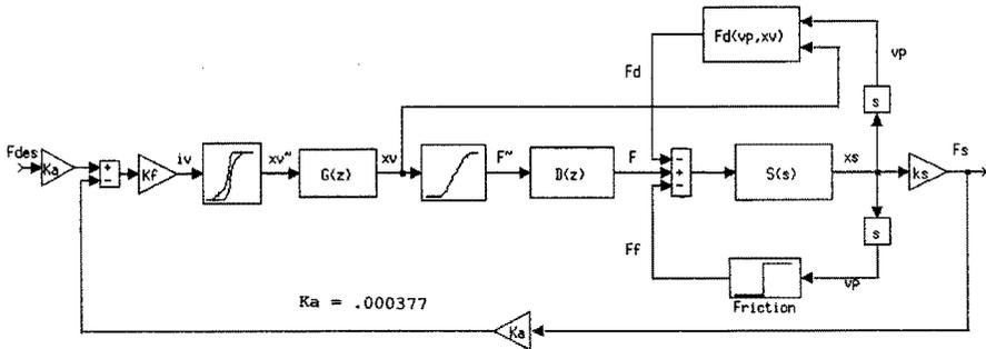
Figure 2: Block Diagram of the Closed-Loop Model
