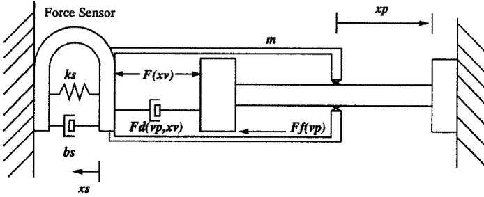
Figure 4: Actuator Model
