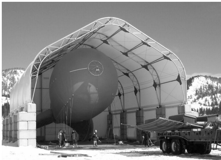
Figure 11: Hangar and tractor-trailer used to house and transport the aerostat.
