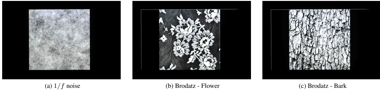
Figure 4: Textures rendered on the display as captured by the camera. For all these images the object to sensor distance is 1.5 m, focus distance 1.22 m, and f/11 with 0.5 s exposure. The captured images are of size 4288 \times 2848 pixels but we only use the center part for our experiments.
