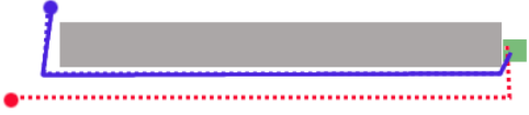
Fig. 1. The follower is blue (solid) and the leader is red (dashed). For appropriate choice of the difference in maximal speeds between the two robots and the weight of the visual occlusion term, the cost of following the shortest path to the common goal (green rectangle) is higher than the cost of going to the other side of the obstacle where the leader is. So, the cost J violates the triangle inequality.
