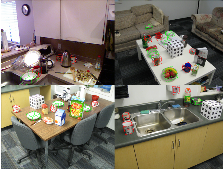
Figure 7.5: Qualitative Parts-Model Results: Sample results of our 3D object detection method, thresholded at 90% precision. The top-left image is from the Kinect sensor, the remainder are robot-collected.
