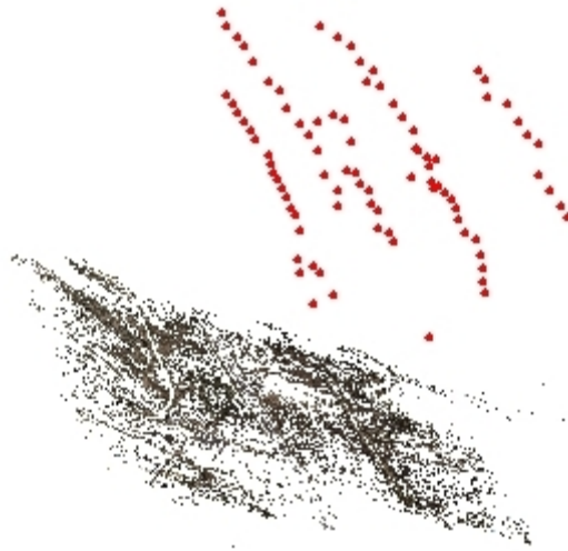
Figure 7- Geometry of final reconstruction for Princeton test data. Sensor positions along 6 flight lines at 2 different flying heights are represented in red with matched ground points shown in their original color.
