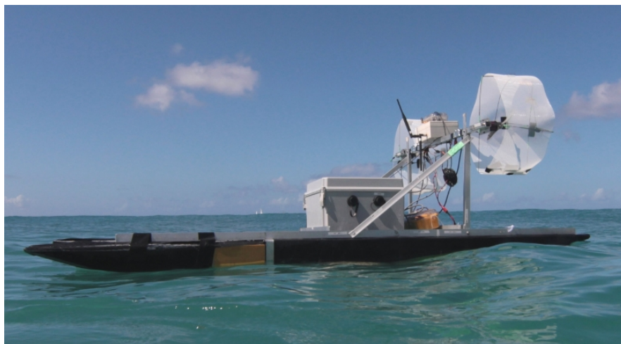
Figure 2.8: MARE is an autonomous airboat made from off-the-shelf components, and is capable of exploring turbulent open water environments. Its discreet air-propelled design and hydro-dynamically stable catamaran hull structure make MARE suitable for long-term deployment in all types of bodies of water. Since it has no moving parts in contact with the water, MARE can explore marine ecosystems while introducing minimal disturbance.
